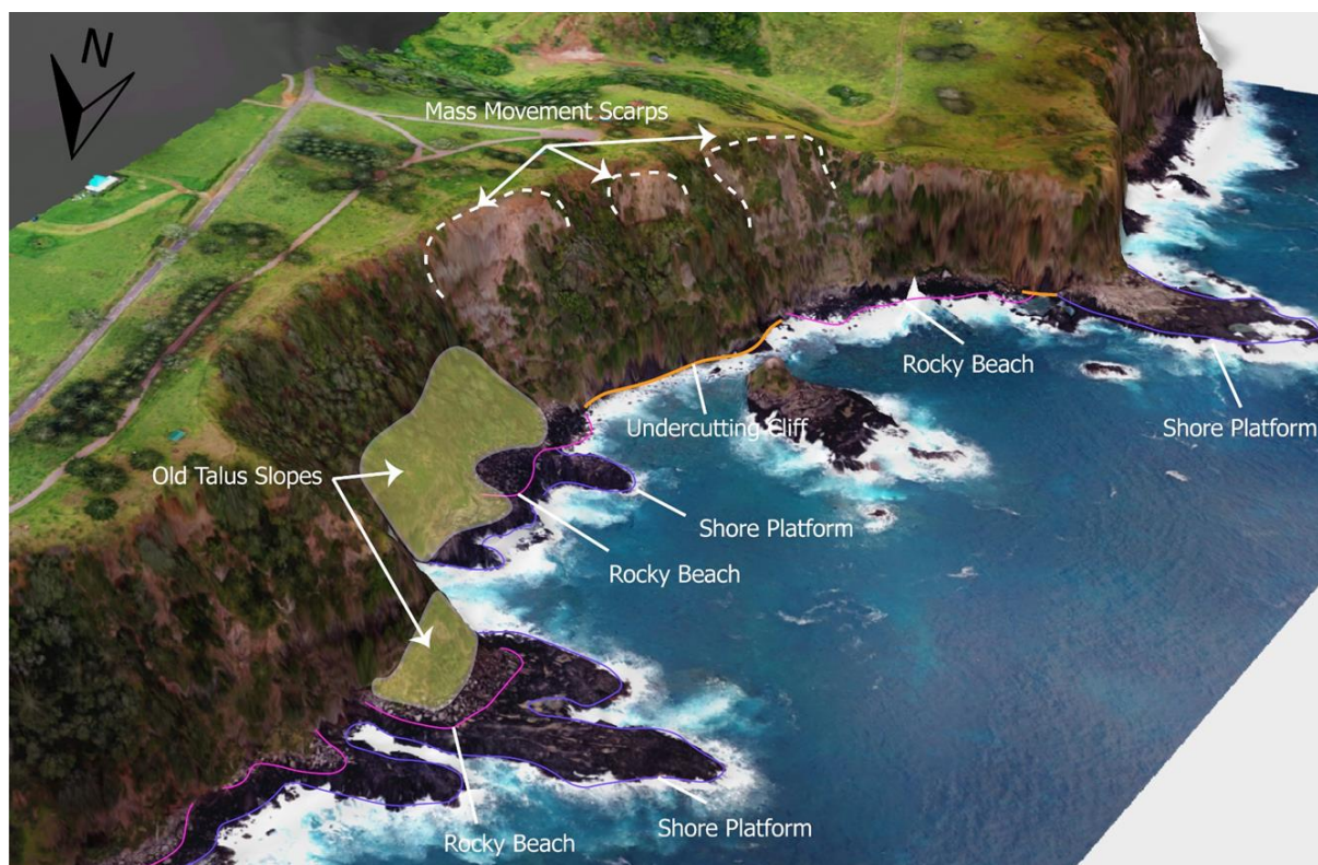
Figure 5-7: 3D drone photogrammetry of Puppy's Point showing mass wasting scarps and old talus slope build up. Platform is alternating shore platform, rocky beach and undercutting cliff.
