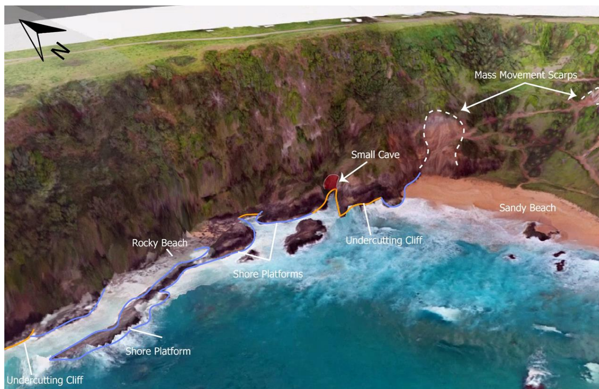
Figure 5-5: 3D drone photogrammetry of the northern end of Anson Bay. The cliff shows evidence of undercutting and formation of small cave between sections of shore platform.
