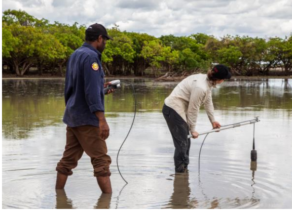
Using a multiprobe to take water quality measurements and recording them in the I-Tracker application
