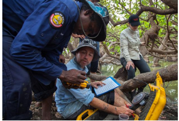
Using a multiprobe to take water quality measurements and recording them in the I-Tracker application
