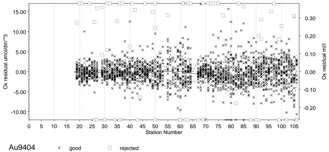
**Figure 5:** Dissolved oxygen residual ( $o_{\text{btl}} - o_{\text{cal}}$ ) versus station number for cruise au9404. The solid line follows the mean residual for each station; the broken lines are  $\pm$  the standard deviation of the residuals for each station (as defined in the CTD methodology).
