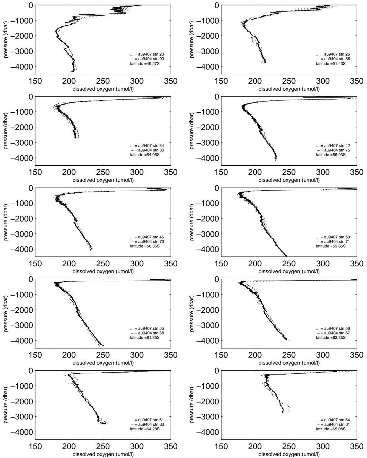
**Figure 7:** CTD dissolved oxygen vertical profile data for comparison of au9404 and au9407 data.
