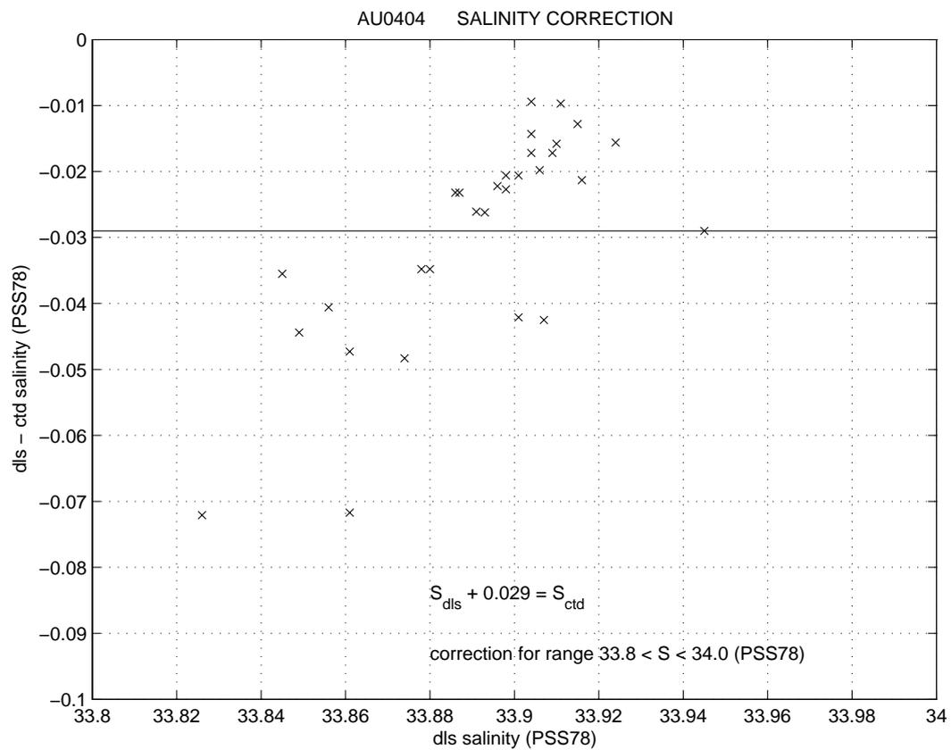
**Figure 6a and b:** Comparison between CTD and underway data, for (a) sea surface temperature, and (b) sea surface salinity. Mean offset value is also shown.
