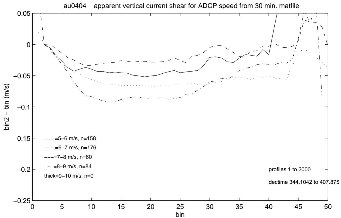
**Figure 5:** Apparent vertical current shear calculated from uncorrected (i.e. ship speed included) ADCP velocities for cruise au0404. Data are divided up into distinct speed classes (i.e. ship speed), shown by the different lines. The top panel shows data for ship speed speed classes from 0 to 5 m/s; the bottom panel is for 5 to 10 m/s. The horizontal axis is vertical profile bin, while the vertical axis is the speed difference between bin 2 and all other vertical bins.
