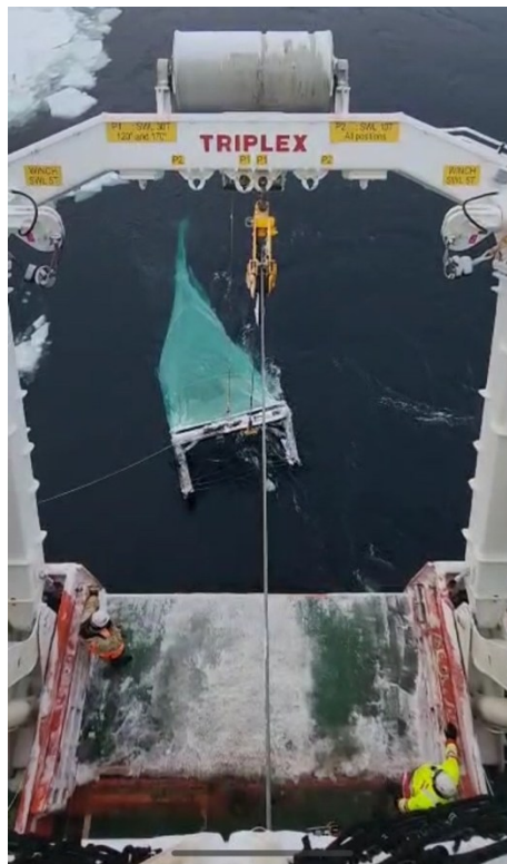
Figure 36: Beam trawl and winch used for all trawls except trawl D, E, F and G, in which the trawl winch was utilised.
