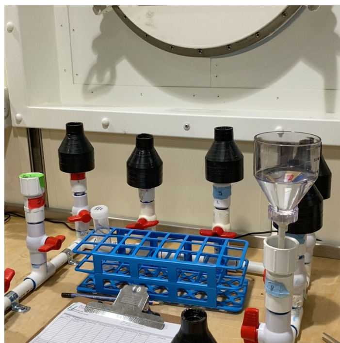
Figure 52: The filtering set up used during the DMV for underway samples.
