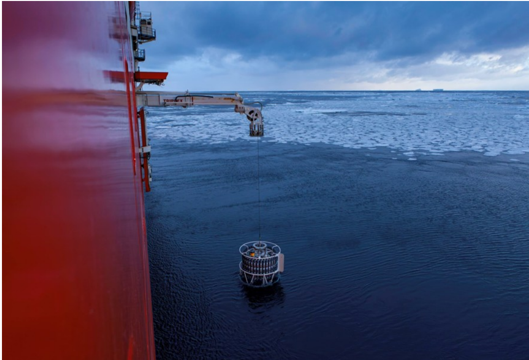
Figure 5. The CTD rosette is deployed from an extendable arm through the side of the ship.
