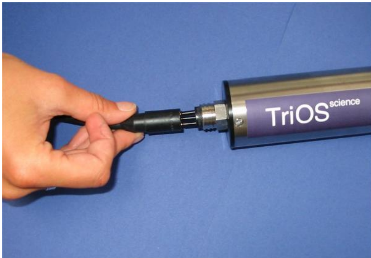
Fig.10 Mounting of the underwater connector
