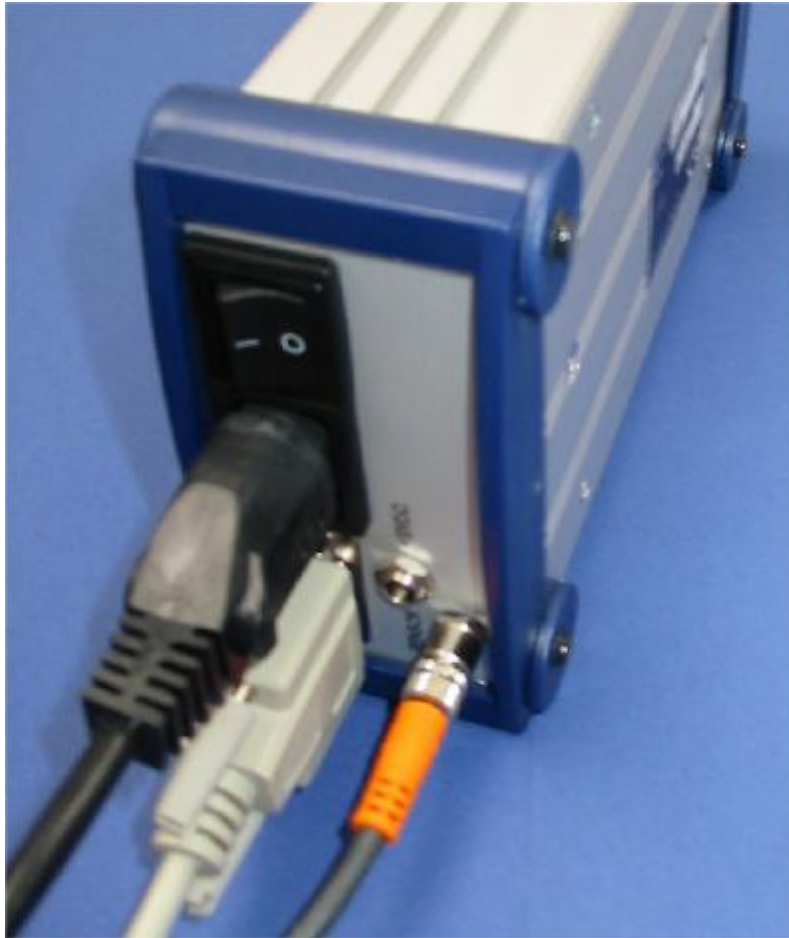
Fig. 13 Connecting the PS101 unit
