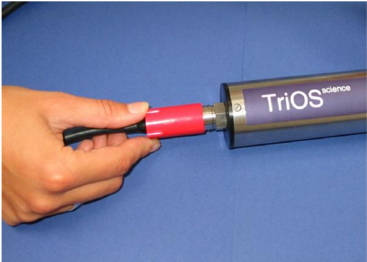
Fig.11 Use of the locking sleeve
