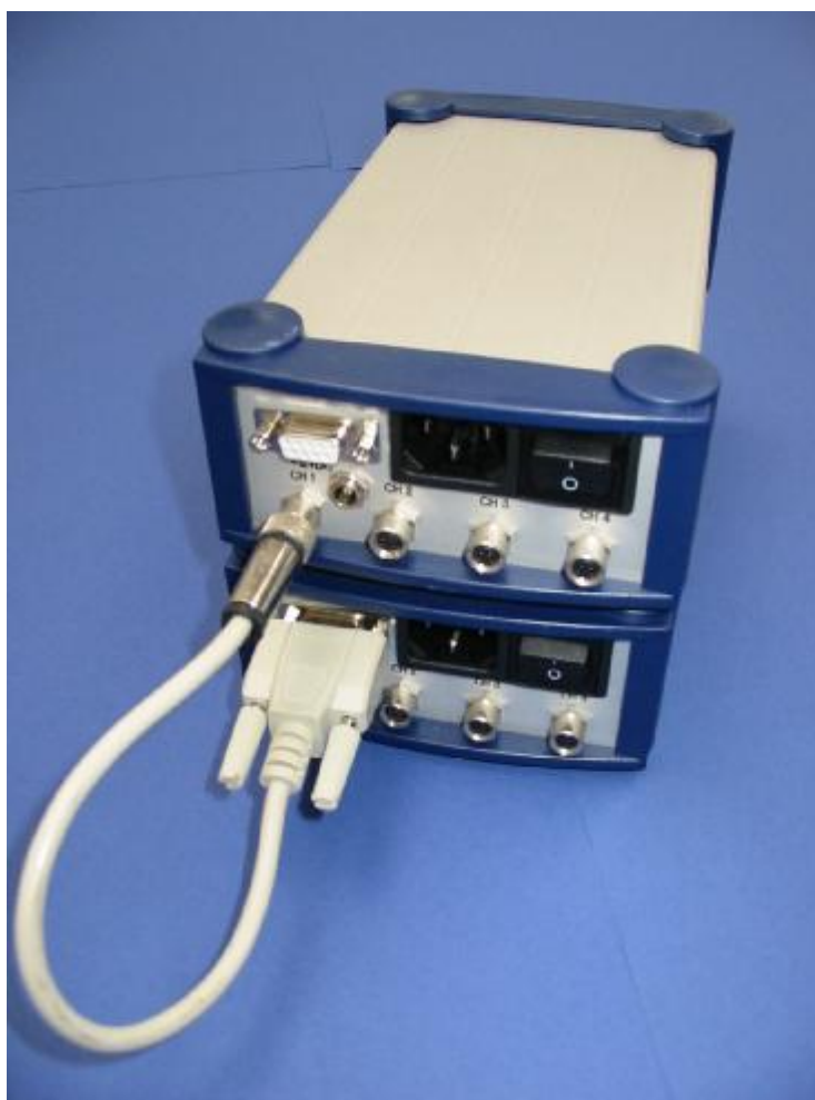
Fig. 14 'stacking' of the IPS104 units to increase the number of connected sensors
