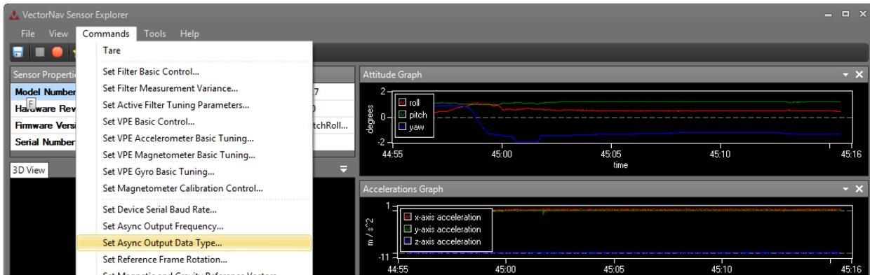
In the **Set Async Output Data Type** dialog box choose **Quaternion, Magnetic, Acceleration, and Angular Rates** and click **OK**.
