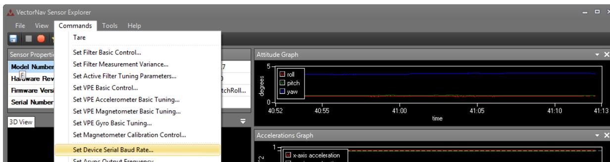
Select baud in the **Set Serial Baud Parameters** dialog box. Make sure that the **Change Sensor Explorer's serial baud rate to match new device baud rate** checkbox is selected and click **OK**.
