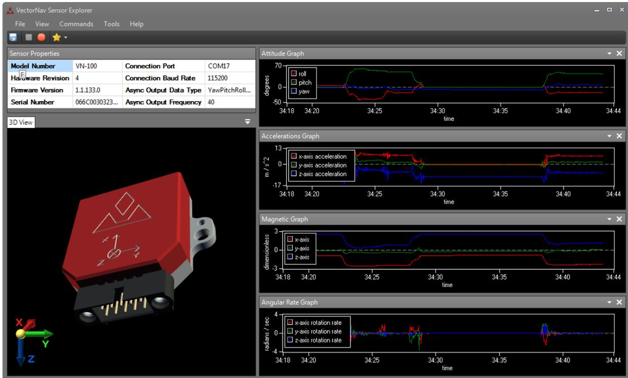
The default parameters for the VN-100 chip are 115200 baud, with Yaw/Pitch/Roll, accelerations, magnetic and angular rates output at 40Hz. As you increase the data output rate or number of output states keep in mind that you will also need to increase the baud rate so that you have sufficient data bandwidth.
