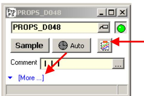
Open the [Advanced Options] by clicking on the small blue arrow at the bottom of the ProPS Control window.
