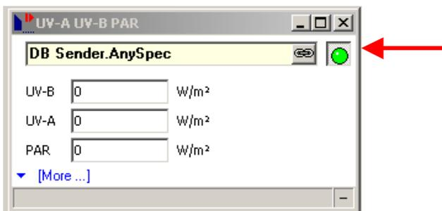
Choose the any spectra of your RAMSES as input (from the DBSender or directly from the RAMSES control)...
