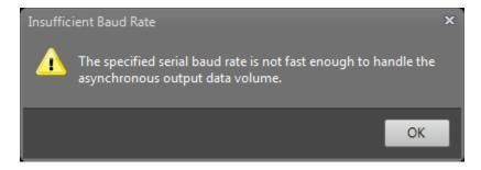
Notice that even though 100Hz was selected from the Command section, the Sensor Properties still reflects 40 Hz in the Async Output Freq (bottom right box). Any time that you increase either the Async Output Freq or change the Async Output Data Type to output more variables than previously displayed always make sure that the baud rate (serial bandwidth) is sufficient to display at your desired settings. In this case since there wasn't sufficient bandwidth, thus the settings did not take effect.
