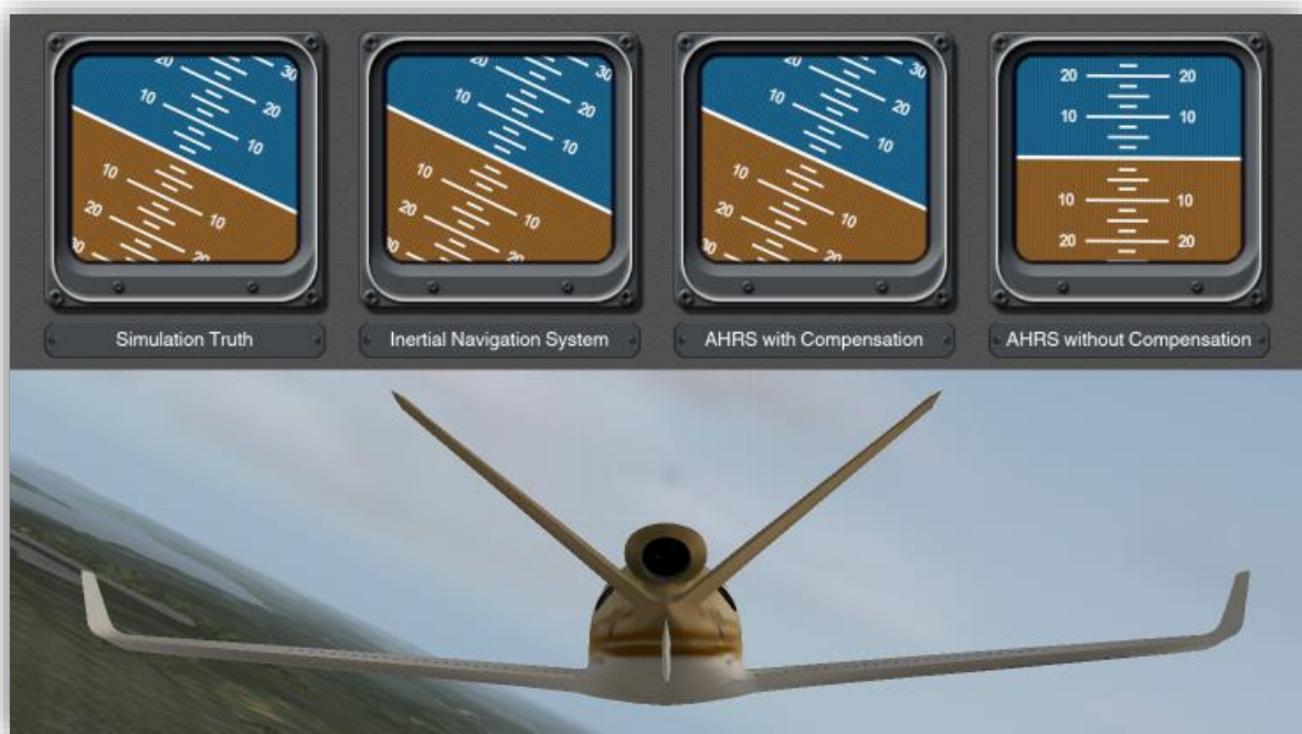
Figure 2 - AHRS with Velocity Compensation
