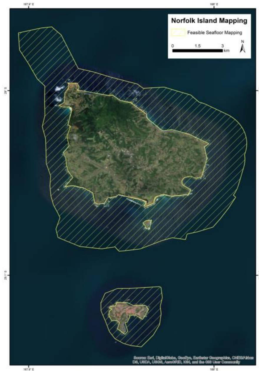
Figure 3: The Area of Interest (yellow) around Norfolk, Phillip and Nepean Islands identified by EOMAP estimated to be optically shallow, i.e., suitable for satellite-based mapping of bathymetry at 2 m resolution.
