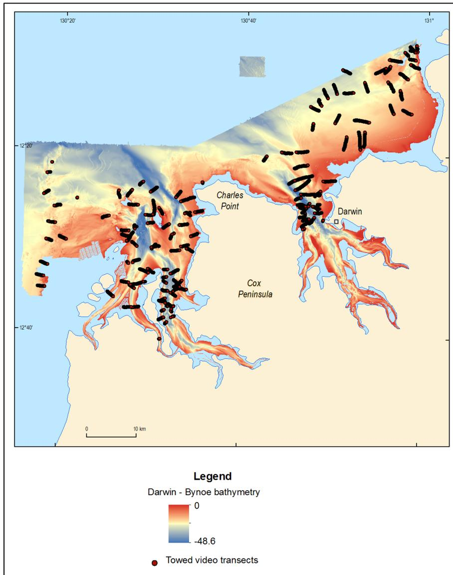
Figure 5. Towed video transects overlaid on multibeam bathymetry grid.
